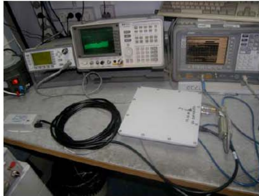
Photo #1. RF conducted emissions test setup.
