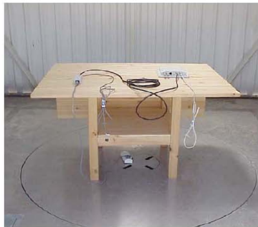
Photo #2. Radiated emissions test setup on OATS.
