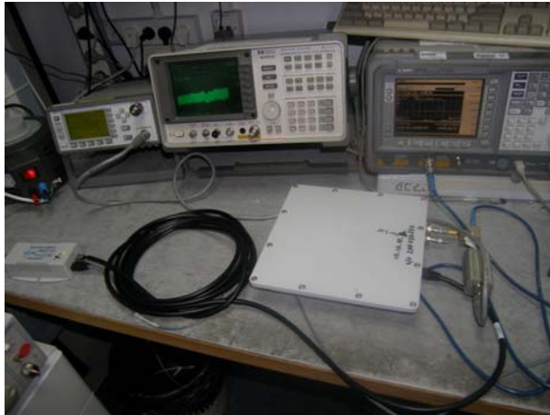
Photo #1. RF conducted emissions test setup.
