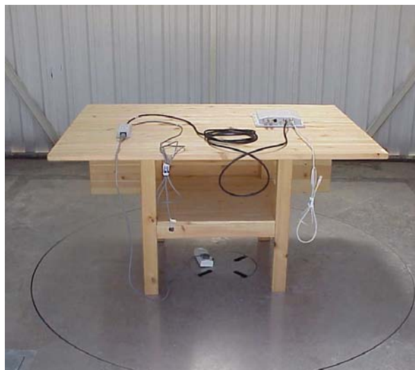
Photo #2. Radiated emissions test setup on OATS.
