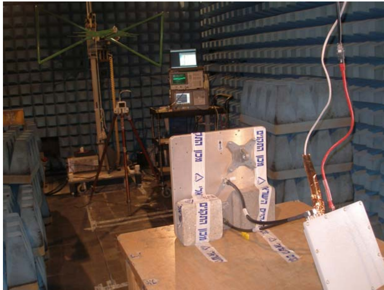
Photo #3. Radiated emissions test setup in anechoic chamber.
