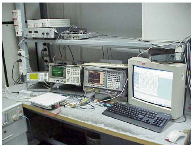
Photo #1. RF conducted emissions test setup.
