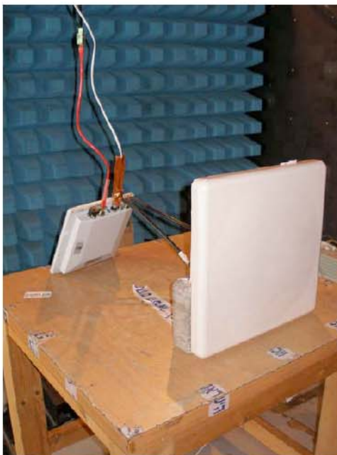
Photo #4. Radiated emissions test setup.
