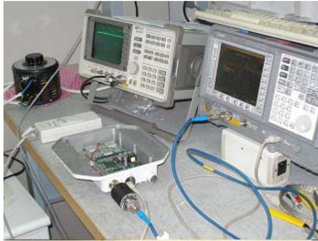
Photo1 Outdoors unit. Test setup
