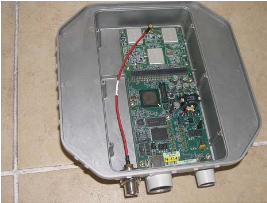
Photo 3 CPE open cover . Components view
