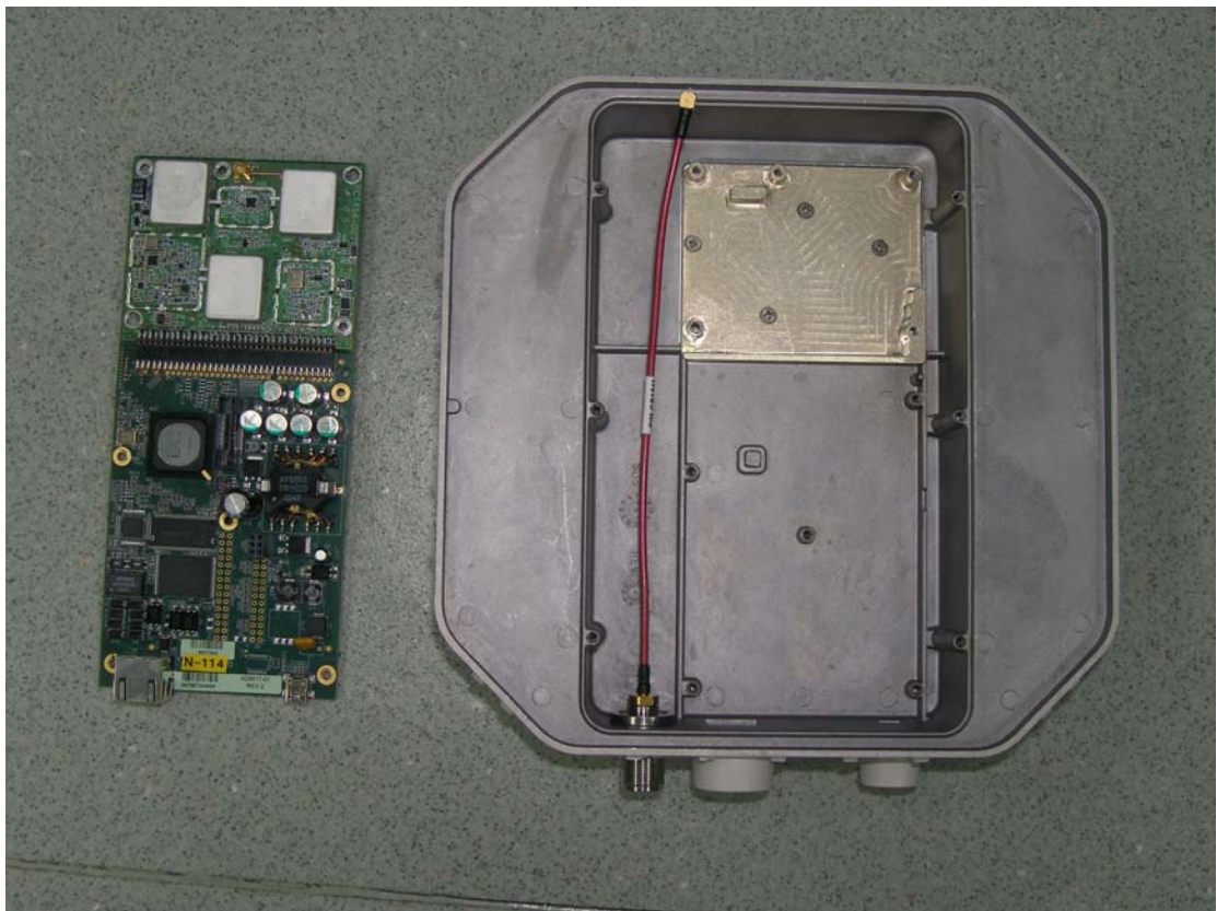
Photo7. CPE with PCB removed , component side
