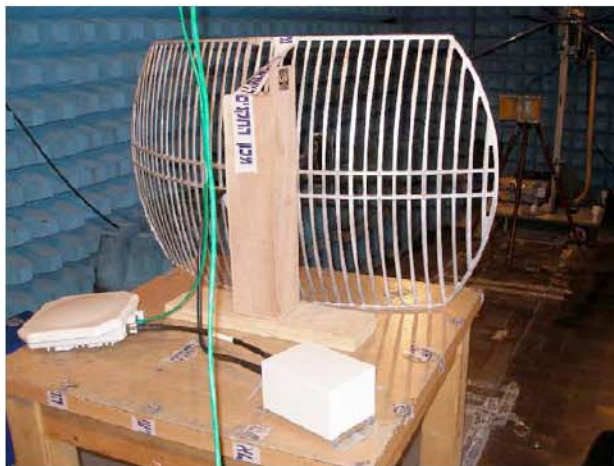
Photo 2. Measurement of radiated emission. Test setup.
