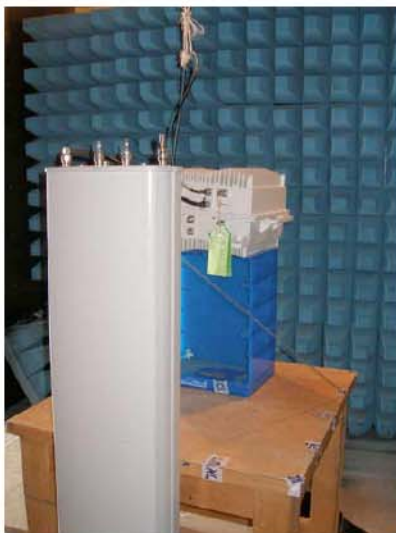
Photo 3. Test setup in anechoic chamber.
