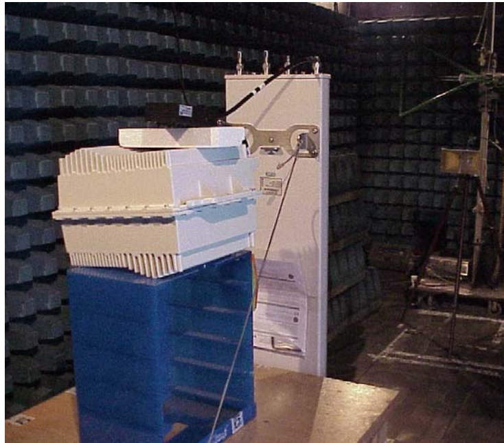
Photo 3. Test setup in anechoic chamber.
