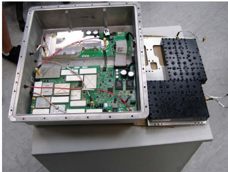
Photo 4. Internal view of outdoor unit.
