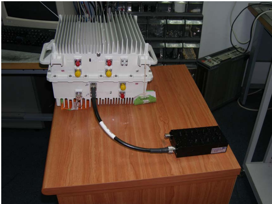
Photo12 . view with external filter
