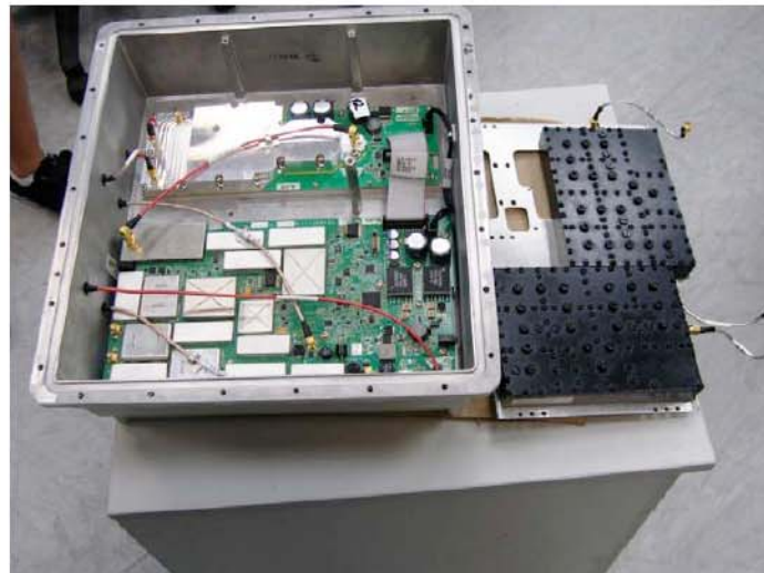
Photo 4. Internal view of outdoor unit.
