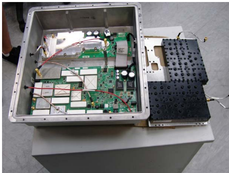
Photo 4. Internal view of outdoor unit.
