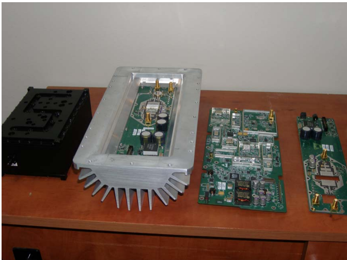
Photo14. From left: cavity filter, open case w/power amplifier PCB, Basic unit PCB, Power amplifier PCB
