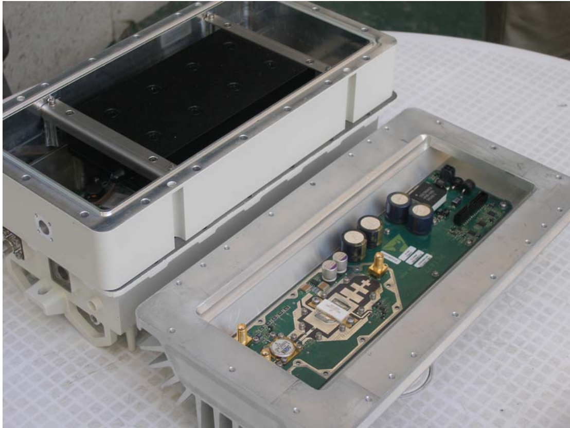
Photo17. ODU open cover , right side Power amplifier
