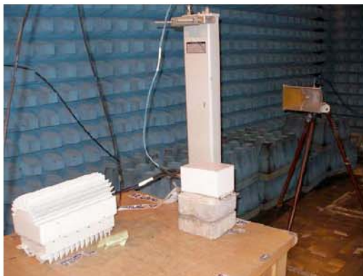
Photo 2. Measurement of radiated emission. Test setup.
