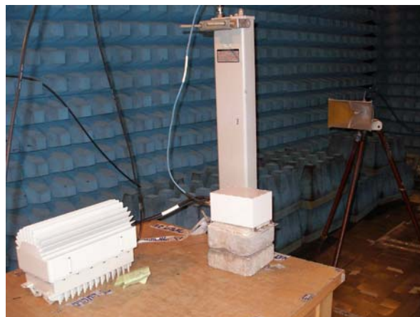
Photo 2. Measurement of radiated emission. Test setup.
