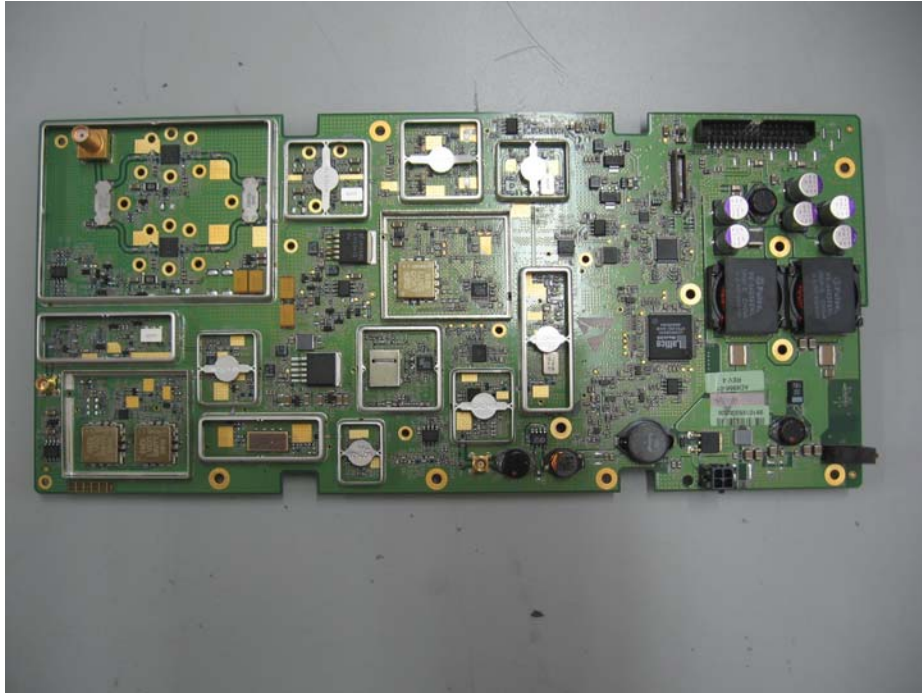
Basic Unit PCB CS Without Cover
