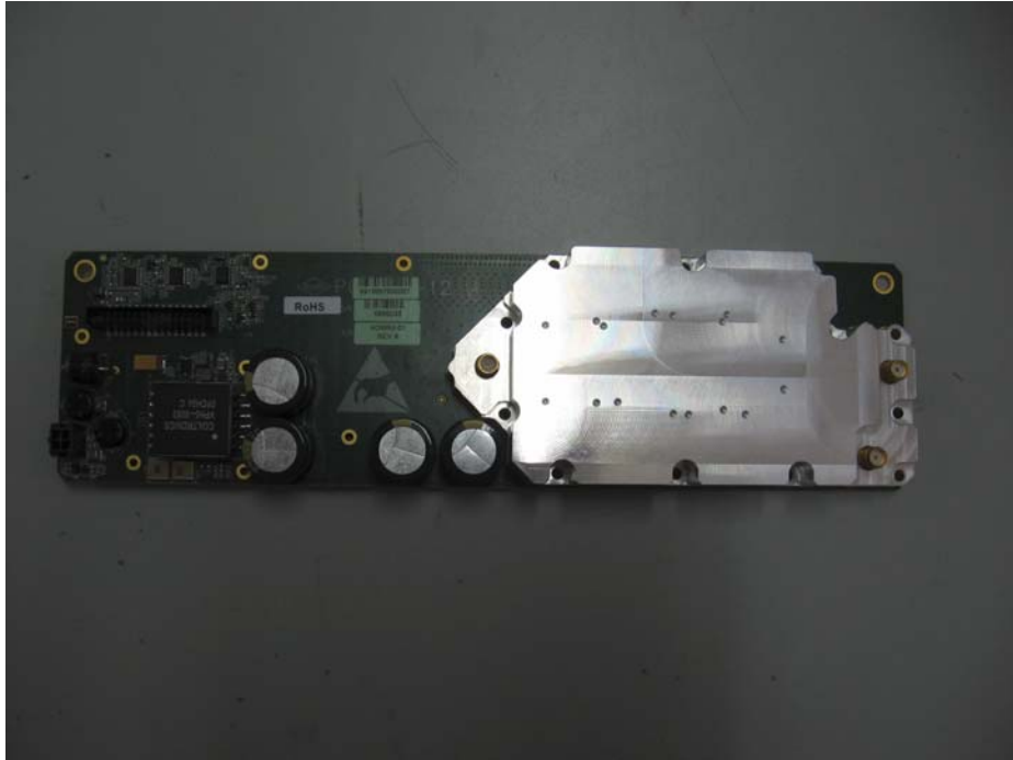
Power Amplifier PCB CS With Temperature Disperse
