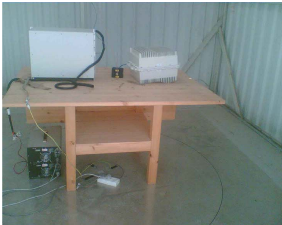
Photos #1-2. Test setup on OATS
