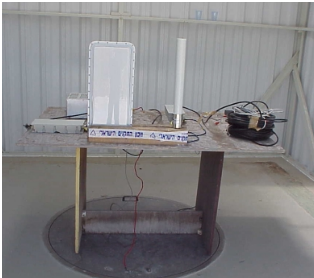
Photo # 6. Base Station + Subscriber Unit Radiated emission test on open site. Front view
