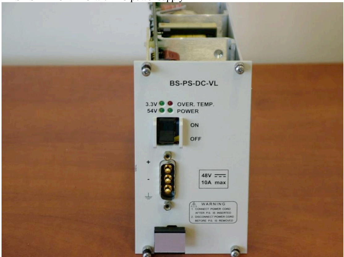
Base station indoor , DC Power supply front panel
