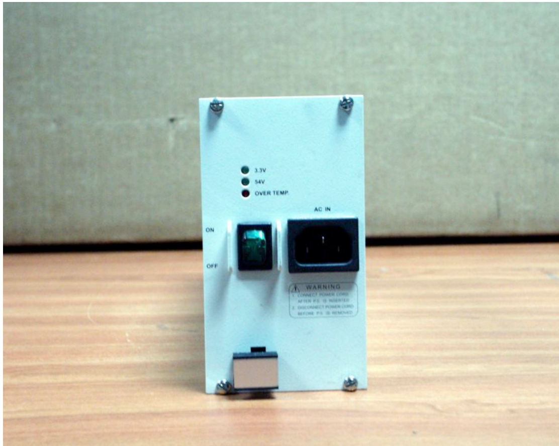
Base station indoor , AC Power supply front
