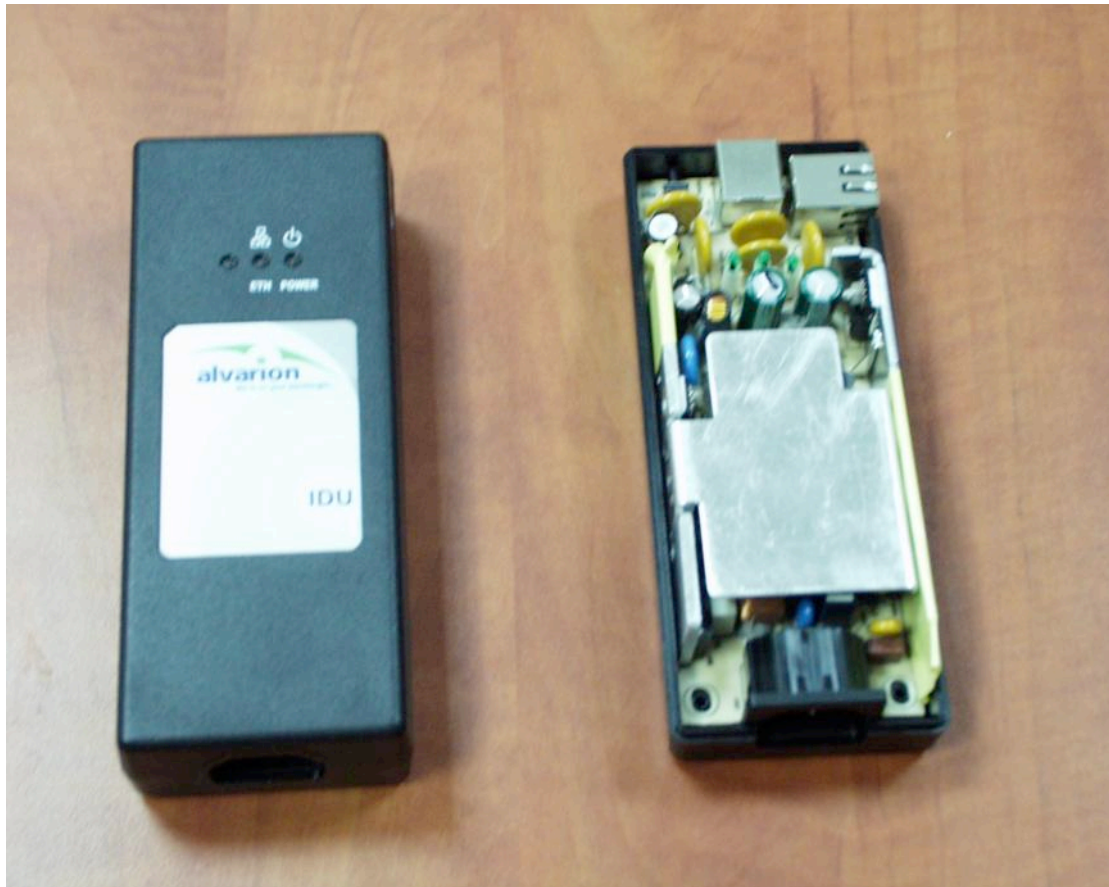
Subscriber unit indoor, top view and cover removed
