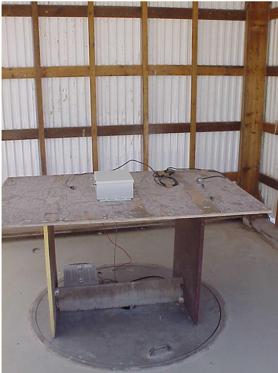
Photo 3. BreezeAccess SU-M-900 Radiated emission test setup at open site
