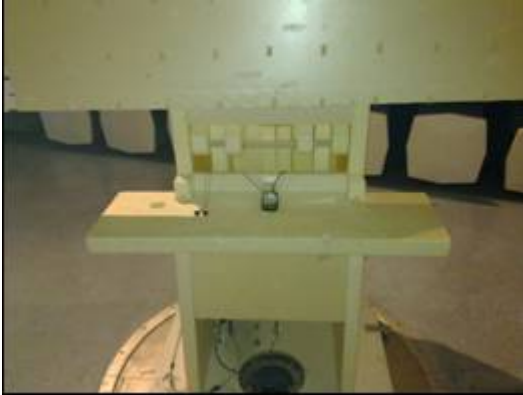
Picture 1. FCC Part 15C Radiated emissions
