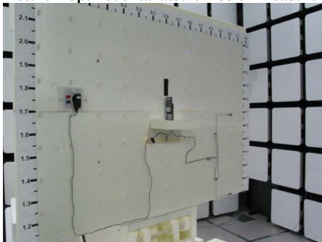
Picture 2 Radiated emission measurement, BT
