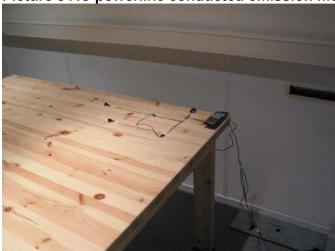
Picture 5 AC powerline conducted emission measurement, GSM
