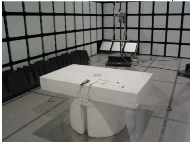
Picture 3 Radiated emission measurement, GSM+FM radio
