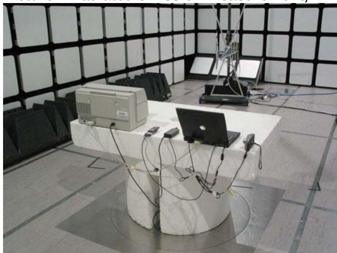
Picture 2 Radiated emission measurement, BT
