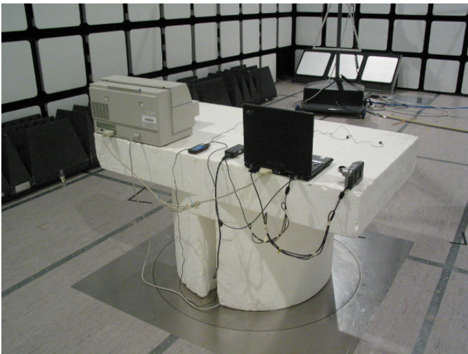
Picture 2 Radiated emission measurement GSM RX / Bluetooth TX / WLAN RX + Computer peripherals
