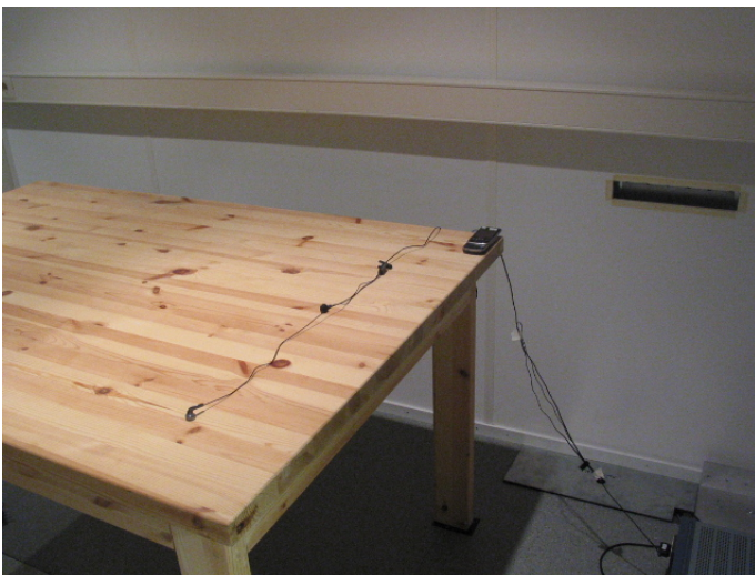
Picture 4 AC powerline conducted emission measurement Bluetooth TX
