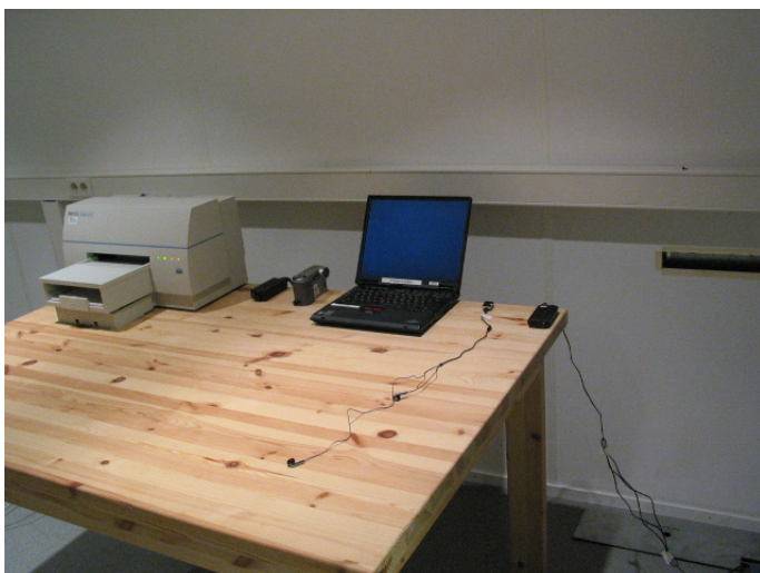
Picture 4 AC powerline conducted emission measurement GSM RX + Computer peripherals
