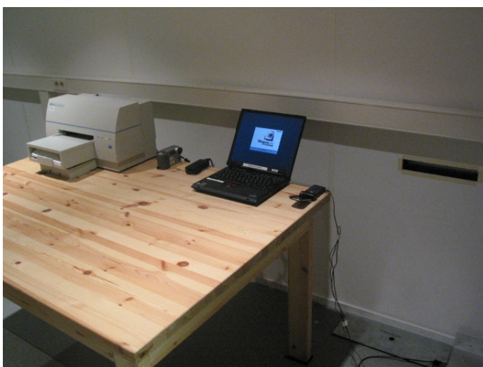
Picture 4 AC powerline conducted emission measurement GSM RX/WLAN TX + Computer peripherals
