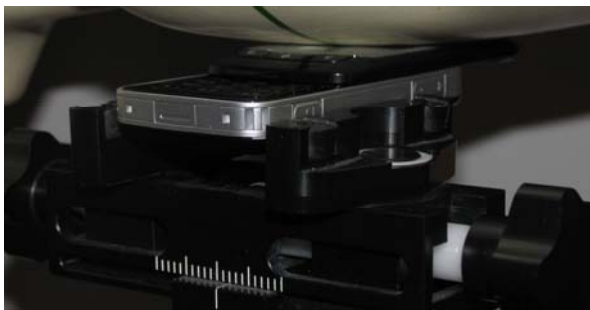
Photo of the device in “cheek” position
