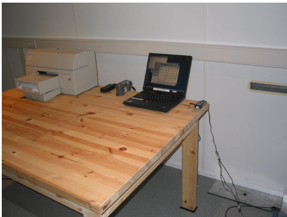
Picture 5 AC powerline conducted emission measurement Bluetooth TX + Computer peripherals
