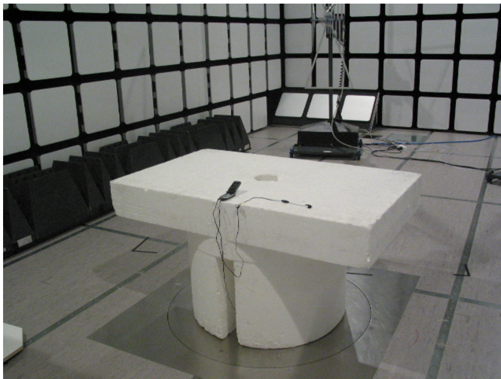
Picture 2 Radiated emission measurement GSM RX + FM radio on
