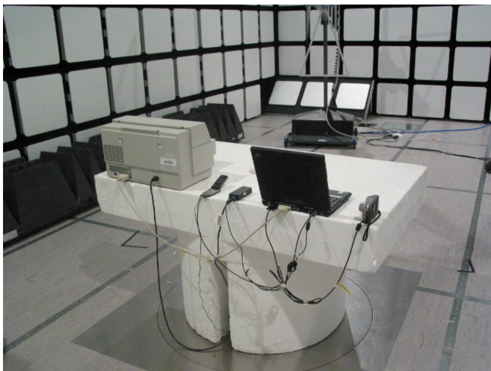
Picture 3 Radiated emission measurement Bluetooth TX + Computer peripherals
