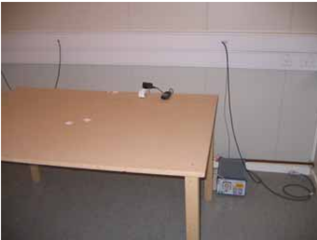
Picture 3 AC powerline conducted emission measurement
