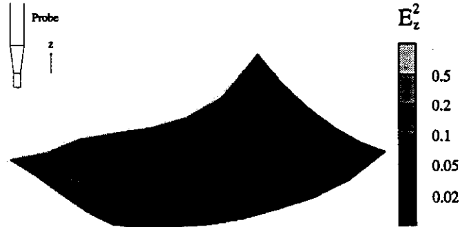
Fig. 9. Distribution of the SAR component in the shell phantom parallel to the probe axis measured with a commercial mobile phone.
