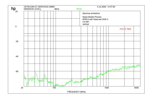
Peaks at 1880 MHz shows the carrier frequency suppressed by narrow band rejection filter
