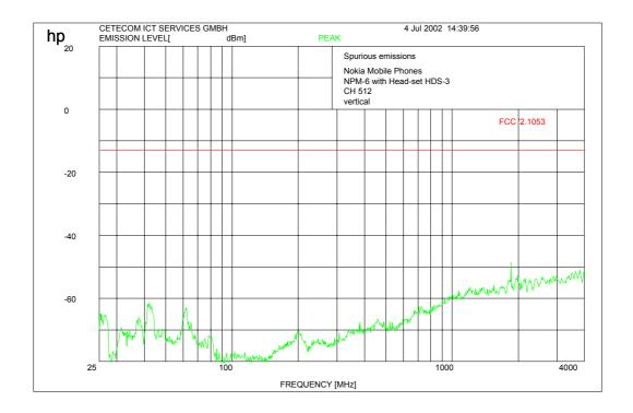
Peaks at 1850.2 MHz shows the carrier frequency suppressed by narrow band rejection filter
