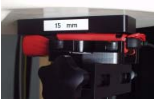
Photo of the device positioned for Body SAR measurement with normal cover and with CC-197D on the left and right, respectively. The spacer was removed for the tests.
