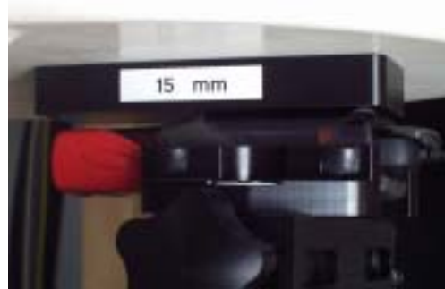
Photo of the device positioned for Body SAR measurement with normal cover and with CC-197D on the left and right, respectively. The spacer was removed for the tests.
