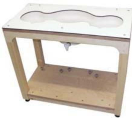
The thickness of phantom shell is 2 mm except for the ear, where an integrated ear spacer provides a 6 mm spacing from the tissue boundary. Manufacturer reports tolerance in shell thickness to be  $\pm 0.1$ mm.
