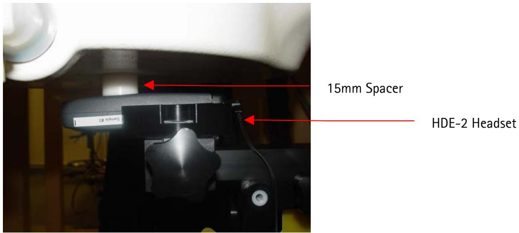
Note: the 15mm spacer was removed before the SAR measurement.
