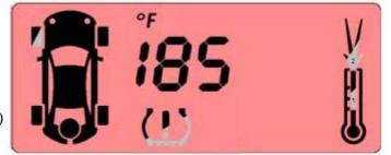
During the alert, the numeric field must display the temperature of the tire and the pressure of the respective tire, cycling for two seconds each. If more than one tire is affected, the system will cycle through the affected tires, displaying each tire information for 2 seconds while reducing the blinking rate of the tires not displayed to 0.5Hz.
