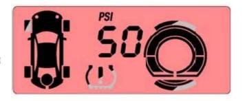
Whenever this condition applies to the spare tire, the "Over Pressure Alarm" icon will be shown and the corresponding icon will blink and beep in the same frequency (1 Hz) for 15 seconds showing the corresponding pressure (only once when ignition is turned on). When all other tires are ok and therefore the corresponding icons are shown continuously, the icon for the spare tire will keep on blinking and the "Over Pressure Alarm" icon will be shown. In spite of the incorrect pressure of the
