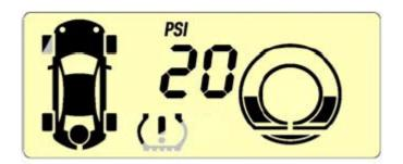
If more than one tire is affected, the system will cycle through the tires affected, showing each under-inflated tire's pressure for 2 seconds continuously.
