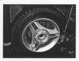
Using the bead buster, bust the inner bead of the tire ensuring no contact is made with the TPMS valve.
