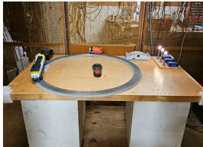
Figure 6: Conducted Emissions Test Setup Photograph(s).
