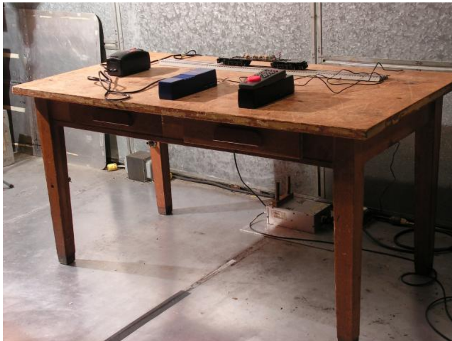
Figure 6: Conducted Emissions Test Setup Photograph(s).
