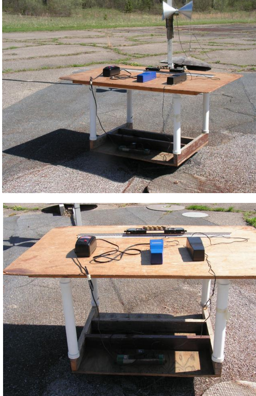
Figure 4: Radiated Emissions Test Setup Photograph(s).
