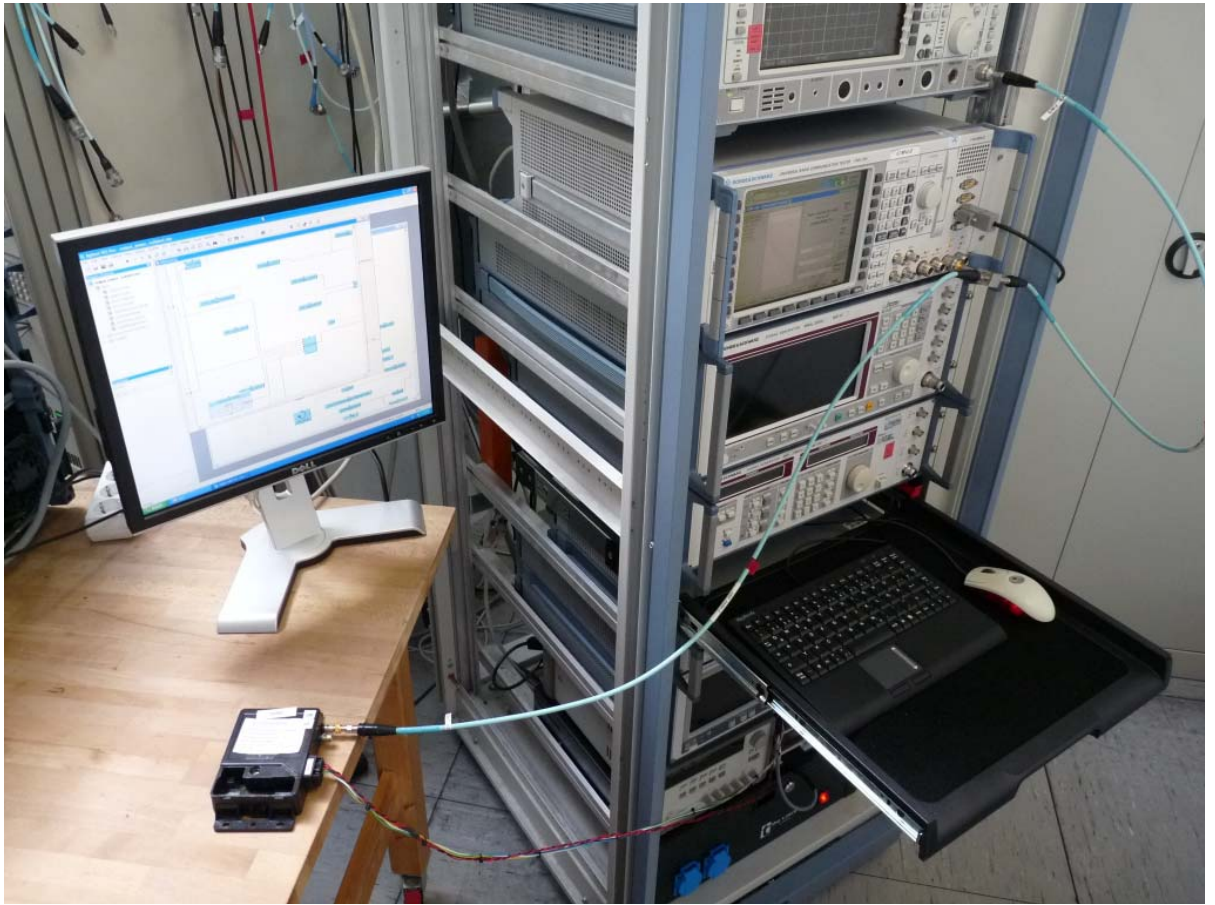
conducted test set-up
