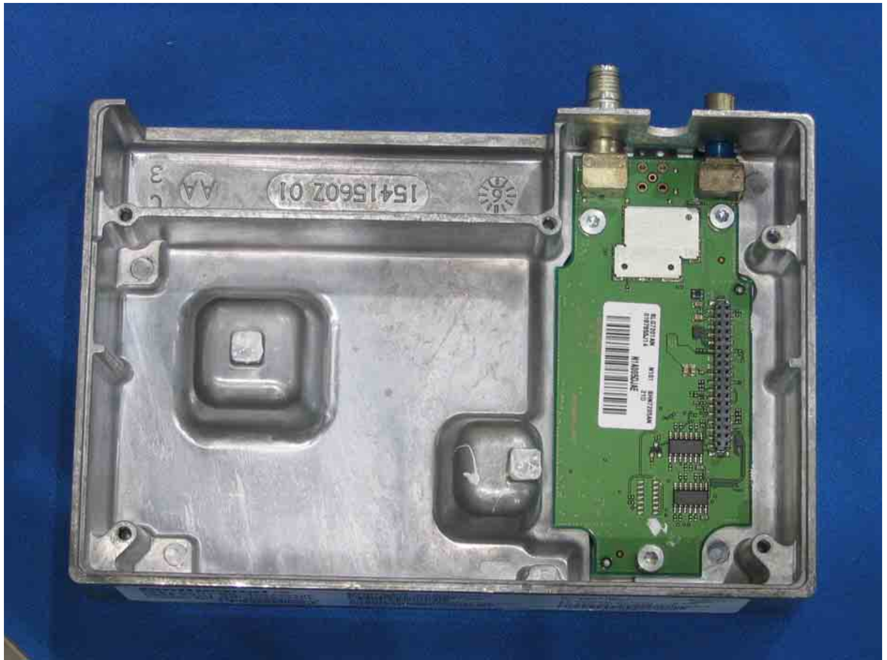
Figure 3: Daughter Board Location in Chassis
