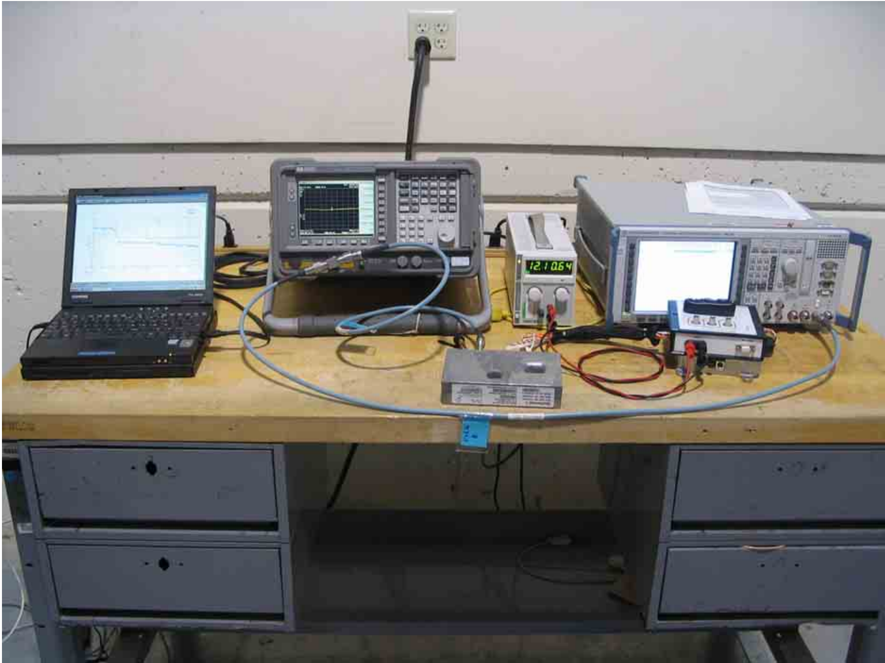
Figure 3: Antenna Terminals Testing
