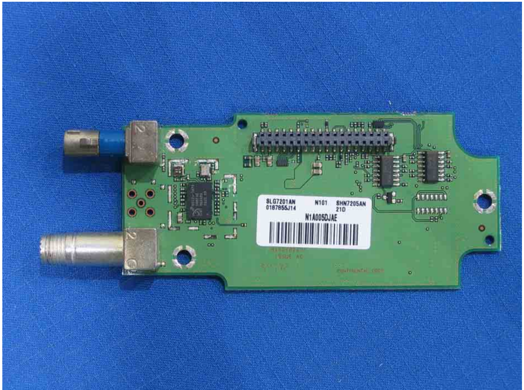
Figure 5: Daughter Board Top Side With Shields Removed
