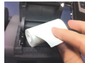
Incorrect roll orientation
