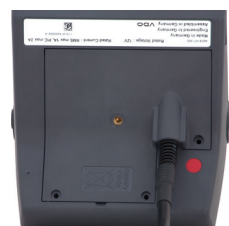
Close the service panel again and insert the three screws included in the box.
