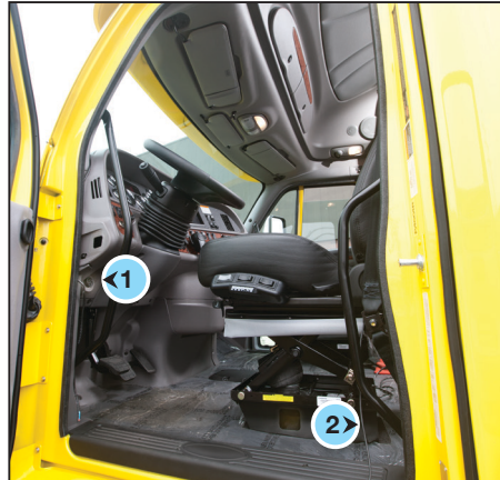
Cable ports are usually located in the dash (1) or on the floor to the left of the driver's seat (2).
