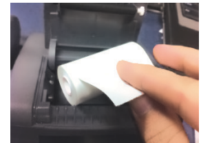
INCORRECT Roll Orientation
