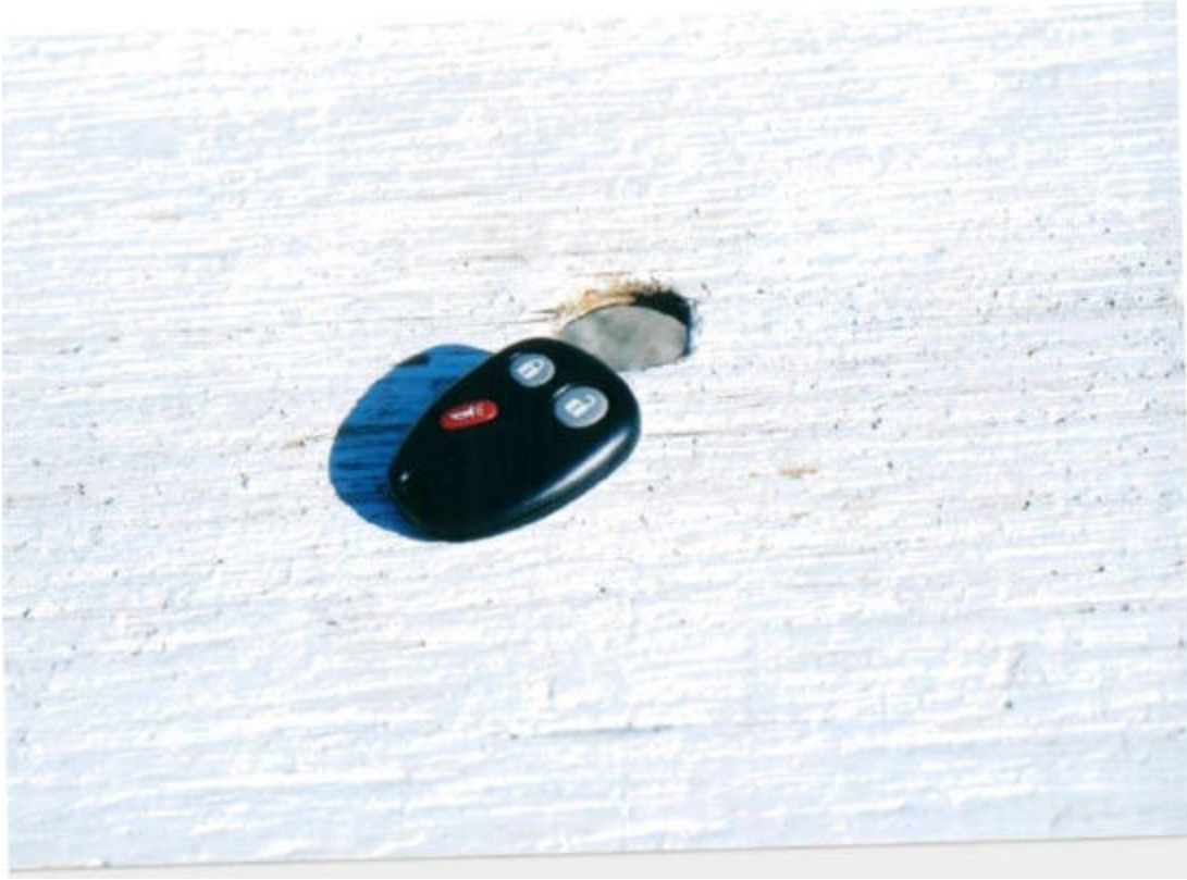
LHJ011 Transmitter Close-Up on OATS
