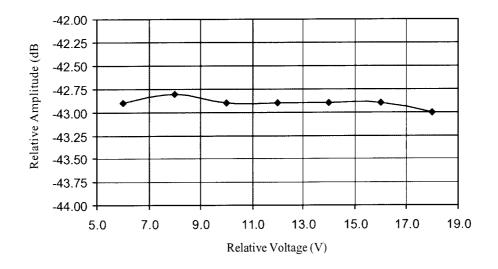
Figure 6.2. Relative emission at "fundamental" vs. supply voltage.
