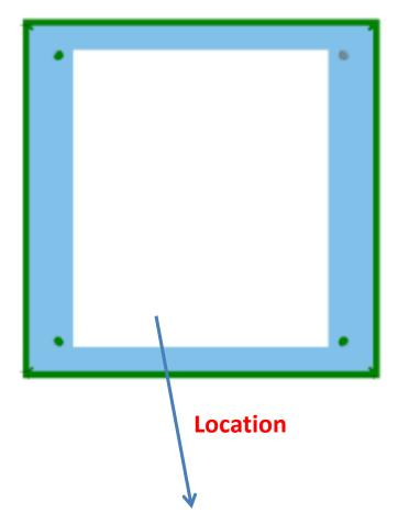
Label with FCC and IC ID information is placed on top of the module and is clearly visible.
