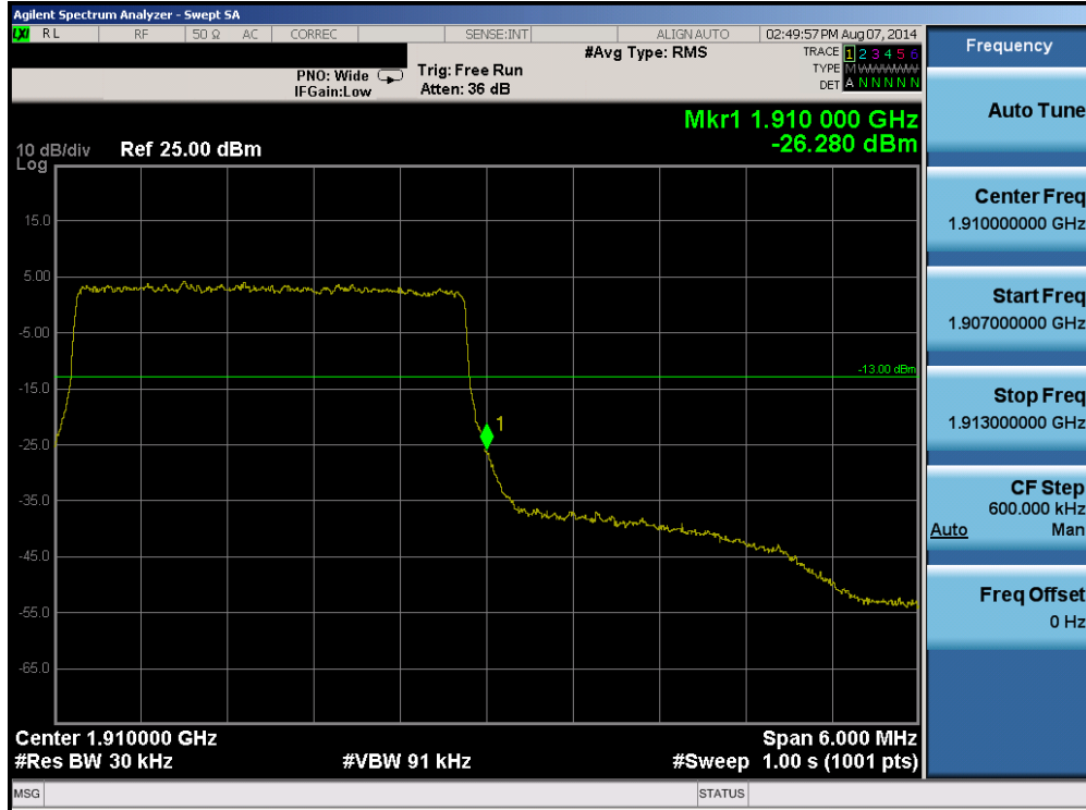
Plot 6-79. Upper Band Edge Plot (Band 2 – 3.0MHz QPSK – RB Size 15)
