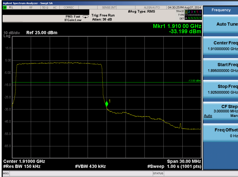
Plot 6-83. Upper Band Edge Plot (Band 2 – 15.0MHz QPSK – RB Size 75)
