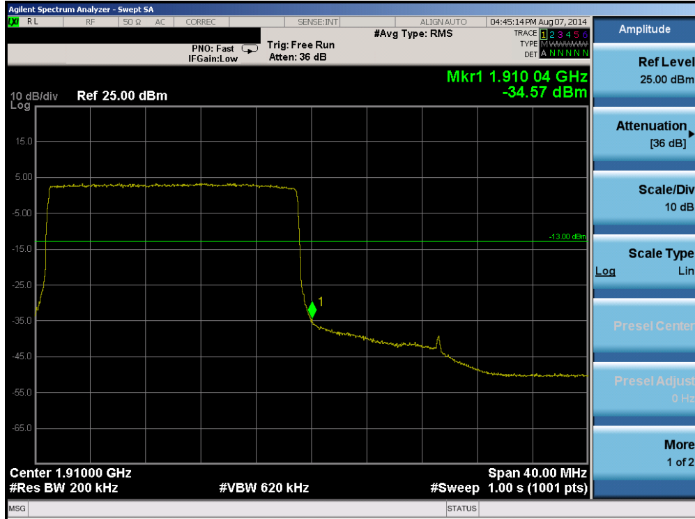
Plot 6-87. Upper Band Edge Plot (Band 2 – 20.0MHz QPSK – RB Size 100)
