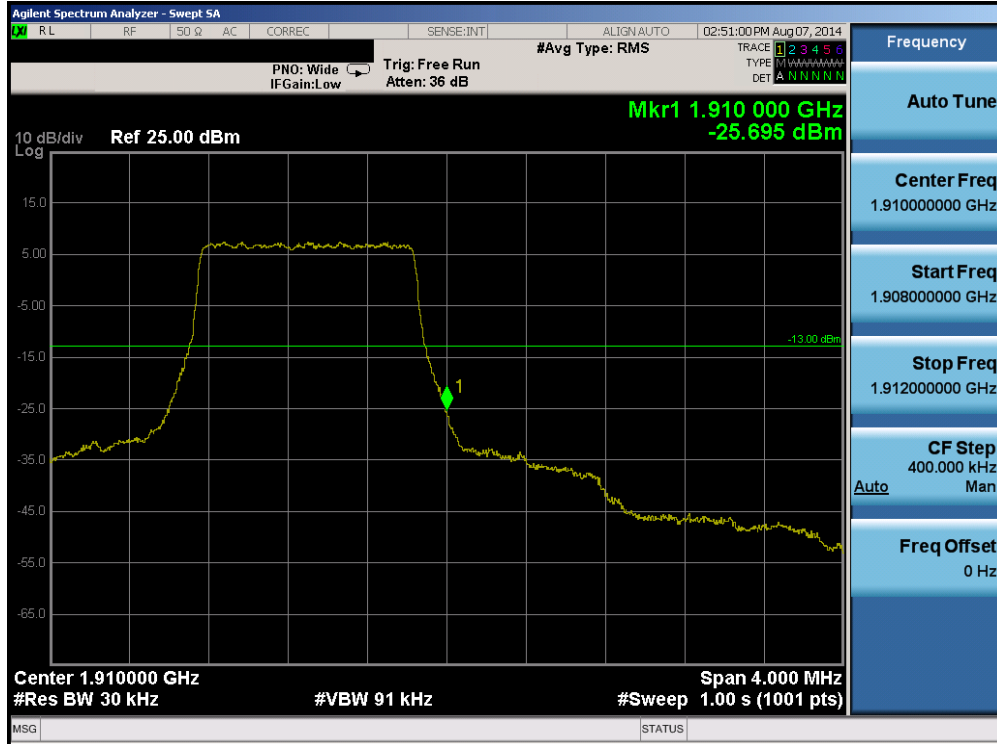
Plot 6-75. Upper Band Edge Plot (Band 2 – 1.4MHz QPSK – RB Size 6)
