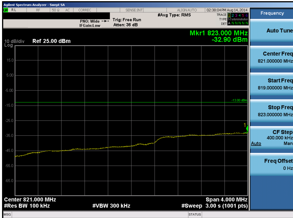
Plot 6-54. Lower Extended Band Edge Plot (Band 5 – 3.0MHz QPSK – RB Size 15)
