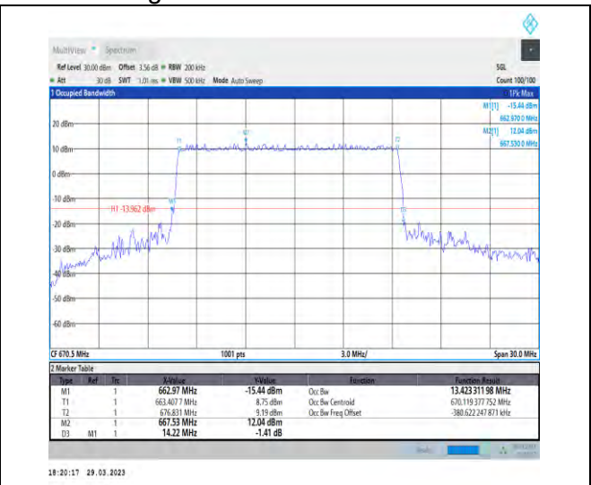
1-N71-15-15-L-4-DFT-64QAM-Outer_Full-75@0-Ant 1-13.423-14.220-≤15-PASS
