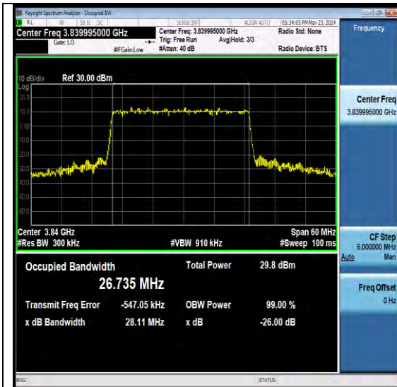
NTNV-N77-3700-3980-PC2-30-30-M-DFT-64QAM -Outer Full-Ant1-PASS
