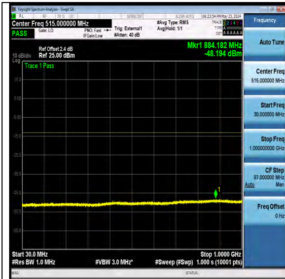
NTNV-N77-3700-3980-PC2-30-100-L-DFT-QPSK-Edge 1RB Left-Ant1-PASS
