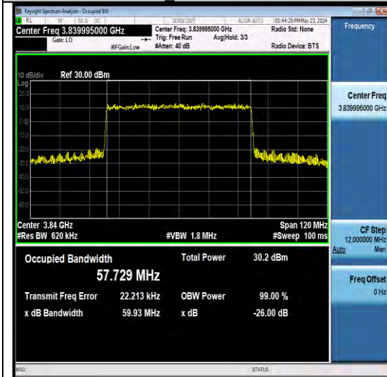
NTNV-N77-3700-3980-PC2-30-60-M-DFT-16QAM -Outer Full-Ant1-PASS
