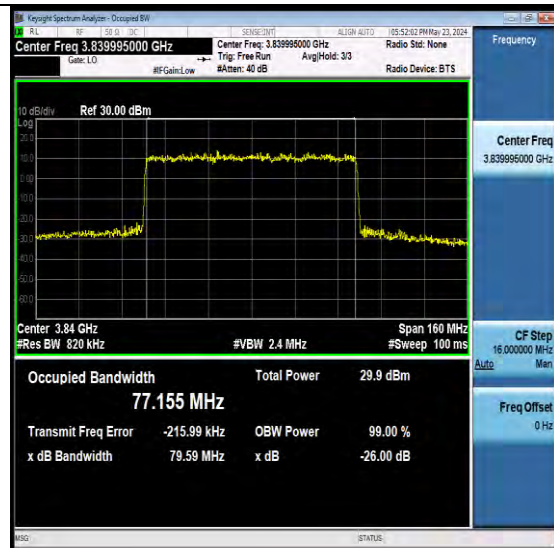
NTNV-N77-3700-3980-PC2-30-80-M-DFT-64QAM -Outer Full-Ant1-PASS
