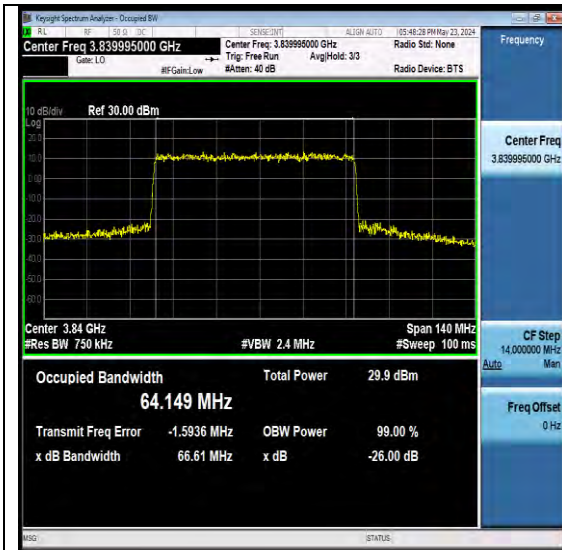
NTNV-N77-3700-3980-PC2-30-70-M-DFT-64QAM -Outer Full-Ant1-PASS
