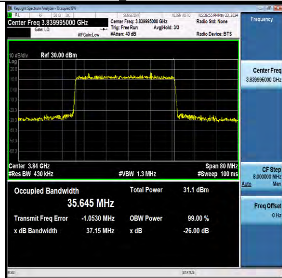
NTNV-N77-3700-3980-PC2-30-40-M-DFT-QPSK- Outer Full-Ant1-PASS
