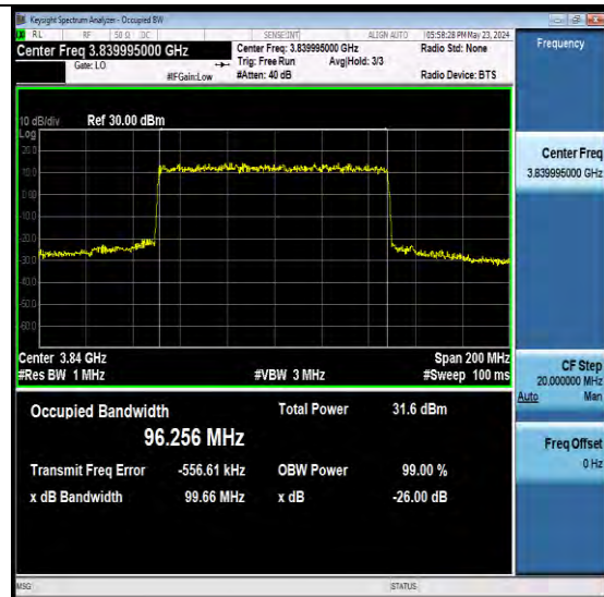
NTNV-N77-3700-3980-PC2-30-100-M-DFT-QPSK -Outer Full-Ant1-PASS
